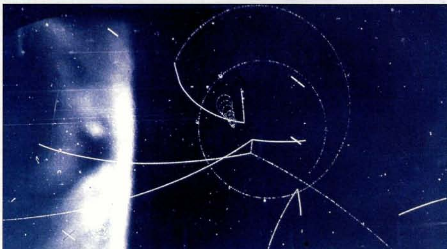
In this image from the Saclay 81 cm bubble chamber, an antiproton (lower of tracks to left) comes in and annihilates with a proton in the liquid, p\bar{p} \rightarrow K^0 K^- \pi^0 . The K^0 moves up the page and decays to \pi^+ \pi^- ; the \pi^+ \rightarrow \mu^+ \rightarrow e^+ decay creates the big spiral track.
