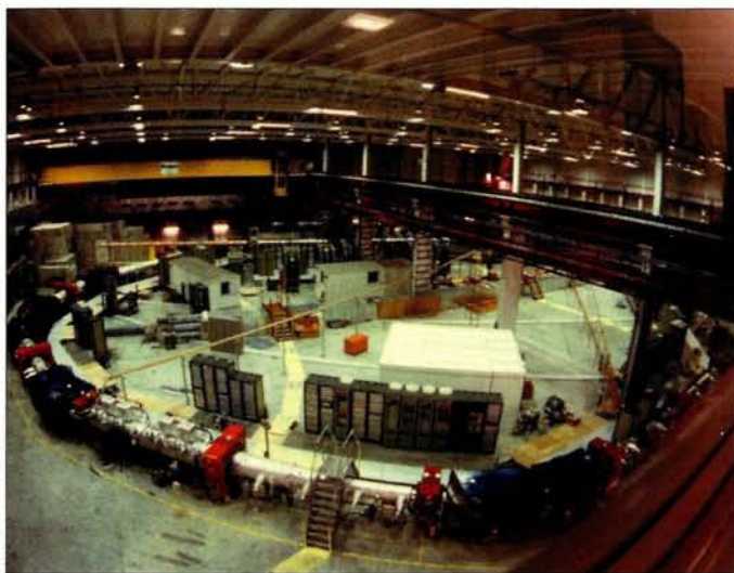
The Antiproton Accumulator, seen here in October 1980, was essential for providing the antiproton beam in the SPS.
